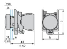
$\boldsymbol{e}$  : clamping thickness: 1 to 6 mm / 0.04 to 0.24 in.  $\boldsymbol{b}$  : 30 mm / 1.18 in.
